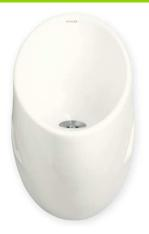
The waterless urinal shall be made of vitreous china. The urinal shall have a 14-3/4" (375 mm) extended rim. The urinal shall include removable strainer, sealing liquid sample, cleaner sample, urinal ball sample, 2" outlet spud, and hangers.
