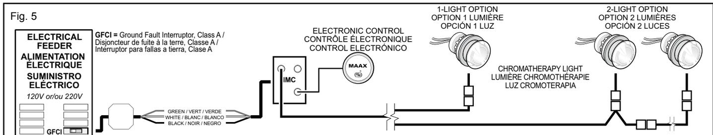
**Note:** Do not use the LOAD wire to connect the light to the electrical box.
