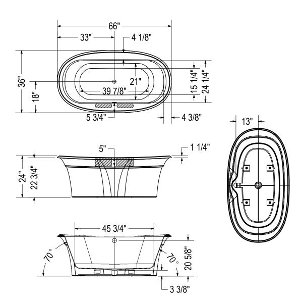
( : Recommended faucet area 2 sections of 10" (L) x 2 1/2" (W) Depth recommended for straight pipes 5".
