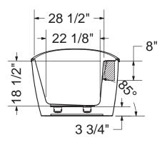
( ( : Recommended faucet area of 15" (L) x 4" (W). Depth recommended for straight pipes 8".
