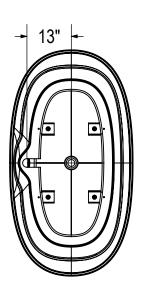
(: Recommended faucet area 2 sections of 10" (L) x 2 1/2" (W) Depth recommended for straight pipes 5".
