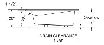
Wood support design may vary. Single Integrated tiling flange: 1" height x 1/4" thickness (shown) Double Integrated tiling flange: 2" height (not shown)
