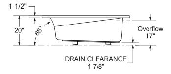
Wood support design may vary. Single Integrated tiling flange: 1" height x 1/4" thickness (not shown)
