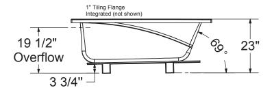
This technical drawing is universal for all ModulR tubs configurations (Drop in, Alcove, IF Corner LH-RH)
