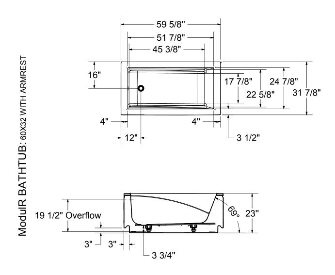
This technical drawing is universal for all ModulR Tub configurations. (Left/Right Corner & Wall-mounted)
