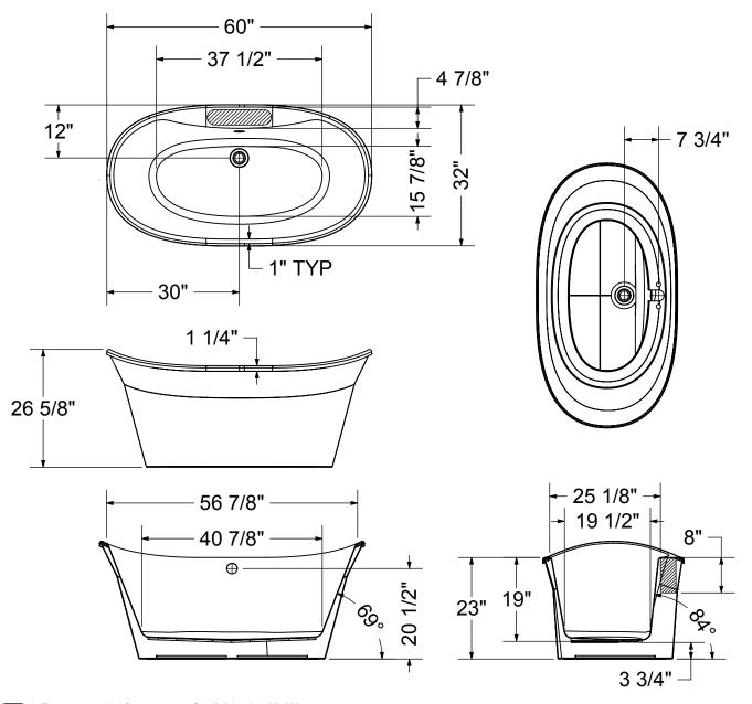
(:): Recommended faucet area of 15" (L) x 3-1/2" (W). Depth recommended for straight pipes 8".
