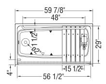
( ▲ ): Indicates Whirlpool jets positioning ( △ ): Indicates suction positioning
