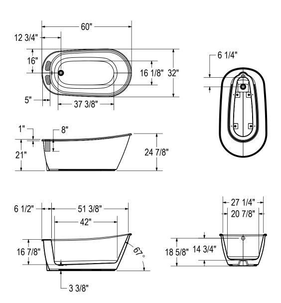
(:): Recommended faucet area 2 sections of 7" (L) x 3" (W). Depth recommended for straight pipes 8".
