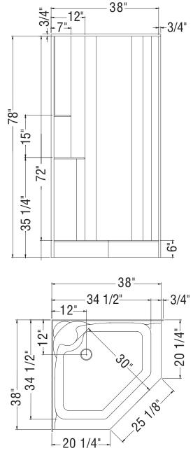
All dimensions are approximate. Structure measurements must be verified against the unit to ensure proper fit.
