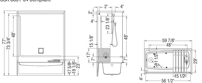
): Indicates Whirlpool jets positioning ): Indicates suction positioning All dimensions are approximate. Structure measurements must be verified against the unit to ensure proper fit.
