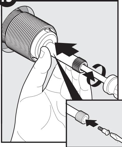
**14** Repeat Steps 7 and 8. If temperature is over ( $>$ ) 120°F, go to 10. If less ( $<$ ) 120°F, turn off flow valve (3 to 6 clockwise) and replace plaster caps.
