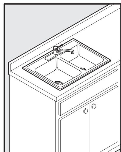
Remove excess caulk and allow caulk to cure following the caulk manufacturer's instructions. Connect faucet to supply lines.
