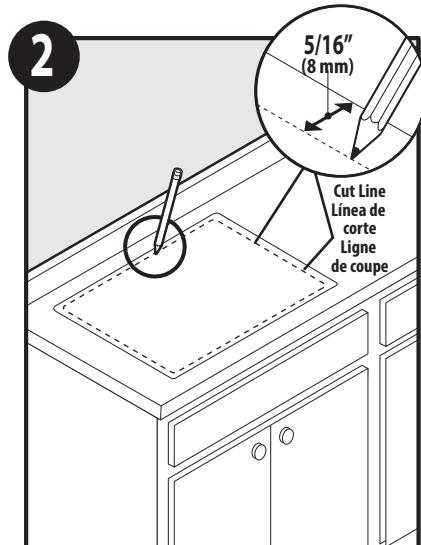
Draw cut line 5/16" inside the sink outline and cut the opening on the cut line.
