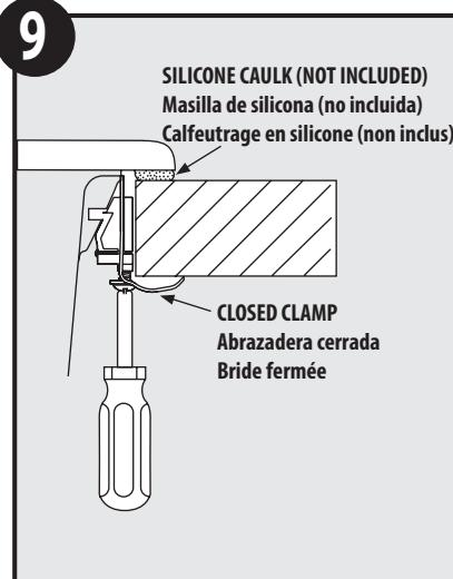
Swing metal portion of clip (clamp) into the clip base. Using a Philips screw driver, turn screw until clamp engages the countertop.
