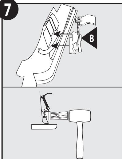
Align clips with corresponding holes in the sink and gently push into place. Push plastic pins in the clips inward completely so that the clips expands and engages the sink. Note that it may be necessary to use a pin punch and hammer to push pin in. Make sure metal portion of the clip (clamp) is in the open position so that the sink can be set into cutout. Proceed to step 8.
