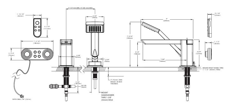
NOTE: THE INSTALLATION SHOWN IS FOR TILE DECKS, THIS VALVE WILL ALSO FIT STEEL, CAST IRON OR PLASTIC DECKS
