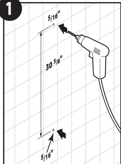
Drill pilot hole to determine if there's a stud. If no wood stud, go to **step 2**. If wood stud, go to **step 3**.
