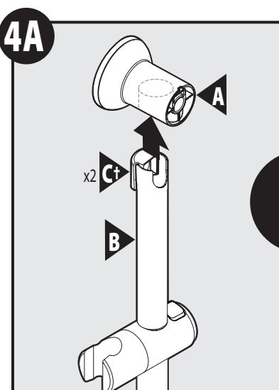
Install Slidebar (B) into each end of Brackets (A). Installation may include Slidebar Caps (C) for certain models.
