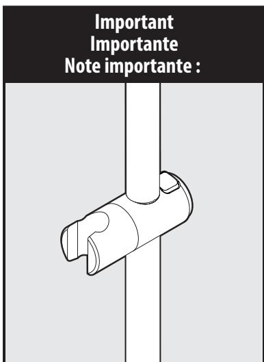
The button on the adjustable slider must be facing up during bracket installation.
