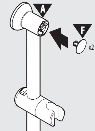
Attach Bracket Caps (F) to Brackets (A), one for each end.
