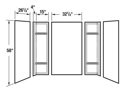
**General:** Furnish and install as shown on plans, DURAWALL® Bathtub Wall model 53, as manufactured by E.L. Mustee & Sons, Inc. The hi-impact thermoplastic wall system shall be 5-piece construction with four formed shelves. One-piece, seamless corner panels with overlapping edges. Uniform color throughout entire thickness of each panel. Color: White.
