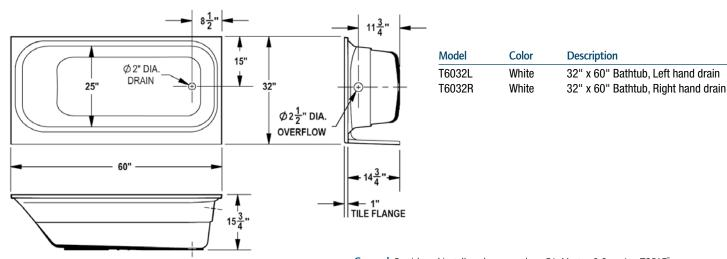
**General:** Furnish and install as shown on plans, E.L. Mustee & Sons, Inc. TOPAZ Fiberglass Bathtub 32"x 60" right or left-handed Model \_\_\_\_\_. Construction shall be molded, reinforced fiberglass using matched metal molds under extreme heat and pressure. Shall meet ANSI Specification Z 124-2017. Color: White.
