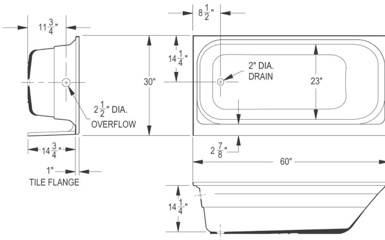
**General:** Furnish and install as shown on plans, TOPAZ® bathtub as manufactured by E.L. Mustee & Sons, Inc. Shall be a fiberglass 30" x 60": right hand or left hand Model \_\_\_\_\_. Construction shall be molded, reinforced fiberglass using matched metal molds under extreme heat and pressure. Shall meet ANSI Specification Z 124-2017. Color: \_\_\_\_\_ (White, Bone, Biscuit) Weight: 55 lbs. Install in compliance with local codes.
