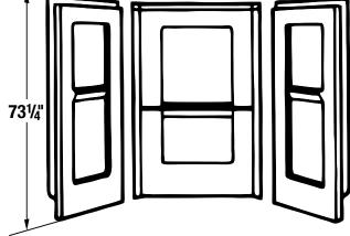
**General:** Furnish and install as shown on plans, 32" square shower, DURAWALL® Shower Walls Model 732, as manufactured by E.L. Mustee & Sons, Inc. Shall be 3-piece, molded fiberglass wall with minimum thickness of 125 mils and mounts direct-to-studwalls. Includes center panel with molded-in shelves and two side panels with molded-in shelf. Self aligning panels use a tongue-and-groove connection. Shall meet ANSI Z 124-2011.2. Color\_\_\_(White, Bone).
