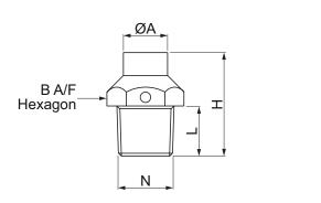
600 PSI Non-Shock Cold Working Pressure to 160°F Maximum Temperature 250°F @ 200 PSI
