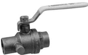
S-FP-600AD-LF - Lead-Free Brass Two-Piece - Full Port with Drain - Dezincification Resistant - Solder NSF/ANSI-61-8, NSF/ANSI-372, IAPMO-IGC-157 - Standard Lever Handle
