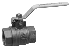
T-FP-600A-LF - Lead-Free Brass Two-Piece - Full Port - Dezincification Resistant - Threaded NSF/ANSI-61-8, NSF/ANSI-372, IAPMO-IGC-157, UL, FM, and CSA** - Standard Lever Handle
