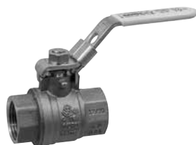
T-FP-600A-LF-LL - Lead-Free Brass Two-Piece - Full Port - Dezincification Resistant - Threaded NSF/ANSI-61-8, NSF/ANSI-372, IAPMO-IGC-157, UL, FM, and CSA** - Locking Lever Handle
