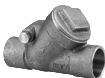
S-413-Y-LF - Lead-Free Performance Bronze™ Check Valve - Solder NSF/ANSI-61-8 (180°F) and NSF/ANSI-372, 200 PSI CWP, Horizontal Swing, Y-Pattern, Integral Seat, TFE Disc
