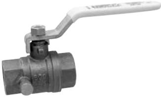
T-FP-600AD-LF - Lead-Free Brass Two-Piece - Full Port with Drain - Dezincification Resistant - Threaded NSF/ANSI-61-8, NSF/ANSI-372, IAPMO-IGC-157 - Standard Lever Handle
