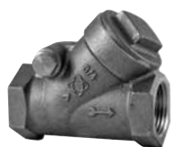
T-413-Y-LF - Lead-Free Performance Bronze™ Check Valve - Threaded NSF/ANSI-61-8 (180°F) and NSF/ANSI-372, 200 PSI CWP, Horizontal Swing, Y-Pattern, Integral Seat, TFE Disc
