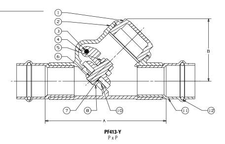
NIBCO® Press System® check valves are designed to meet MSS SP-80 with the exception of the end connection. Male and female press-to-connect ends are new technology not yet covered in the current edition of this specification.
