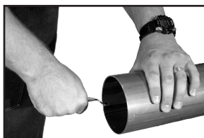
Figure 3: Deburr inside diameter deburring tool
