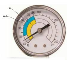
1/2 to 85 psi when testing with air. After ensuring that all connections have been correctly pressed, installers may increase the test pressure to full system test requirements.
