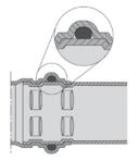
Viega fittings are pressed before, after and on top of the sealing element (3) in a single step which creates a permanent connection that is secure and guaranteed to last.
