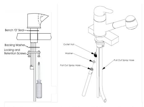
Note: This mixer fits a maximum bench thickness of 2 1/4 inches and has a  $140^{\circ}$  spout arc.
