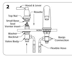
Sidevalve to be installed from underside of work surface as shown.
