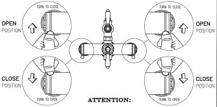
Stop is for temporary use only. Do not leave valve unattended when stop is in the off position. If leaking, rotate stop one full turn to lubricate the stop. A drip in the off position is common. Call 800.777.9762 if problem persists. Do not replace the valve. The stop valve can be replaced if the problem does not stop in the open position.
