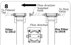
Tighten the hoses from the stop valve to the housings following the flow of the water shown on the cap. When installing the Pre-filter the system flows from the stop valve to the Pre-filter and on to the filter housing and then up to the filter tap.
