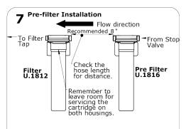
If installing a Pre-filter follow steps 1-3 for the second bracket taking into account the hose length supplied from the Pre-filter to the filter.
