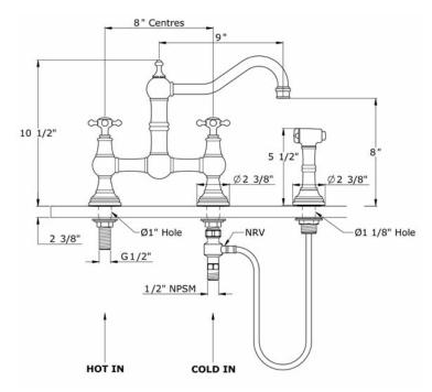
\* For CA/VT, place a "-2" at end of model number for code compliant product. (Example A3608LMAPC-2)
