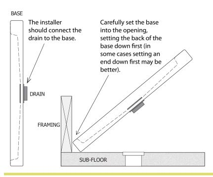
Carefully lower the base down into place, joining the base drain and the floor drain.
