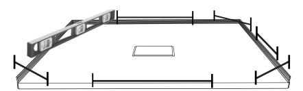
7. After the Installer has connected the drain, the substrate material (sheet-rock, etc.) is ready to be installed. Set your substrate on top of Aluminum flanges (aluminum flanges not intended to be screwed into the studs)
