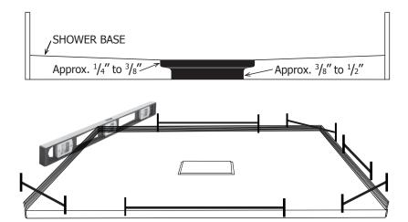
7. After the Installer has connected the drain, the substrate material (sheet-rock, etc.) is ready to be installed. Set your substrate on top of Aluminum flanges (aluminum flanges not intended to be screwed into the studs)
