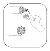
B: Remove restrictor, to increase water pressure, simply take the restrictor out from the shower head handle, see below steps;Carefully pry the restrictor out using a pair of tweezers, a paperclip or a small nail/screw.
