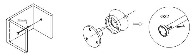
Step 3: Fix and tighten 25 mm tube.
