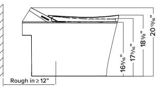
This toilet is designed to rough-in at a minimum dimension of 12" from finished wall to C/L of outlet. Supply not included with fixture and must be ordered separately.
