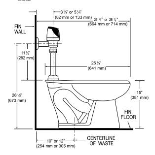
NOTE: All vitreous china dimensions shown in these drawings are nominal. Dimensions can vary within the tolerances established in the governing ASME A112.19.2/CSA B45.1 standard. Please take this into consideration when planning rough-in and plumbing layouts.
