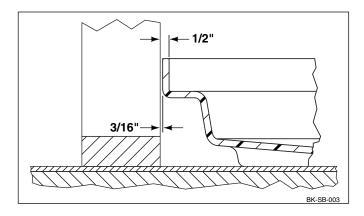
**Note**: When constructing or modifying stud wall framework, make sure to install (gang) multiple studs to provide support for any required moisture resistant wall board, solid surface panel attachment flanges, or filler boards, etc. Framework depth (B) must be at least 3/16" more than the actual depth measurement of the shower floor.
