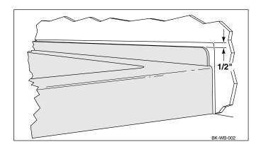
3. The Swanstone or alternate shower wall material will be installed over the 1/2" moisture-resistant wall board and shower floor flange, as shown in the illustration below.
