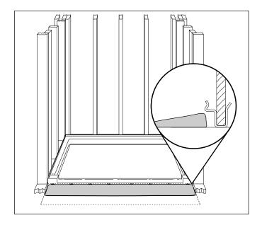
Apply a bead of 100% silicone sealant to seal the joint between the shower floor and shower floor ramp.
