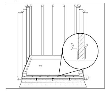
Level the barrier-free shower floor in both directions and make sure all support ribs and the front edge of the shower base make firm contact with the subfloor. If any part of the shower floor is not completely supported, proceed to Steps 5a through 5d; if it is fully supported, skip Step 5.
