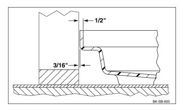
2. After the shower floor installation is complete, install 1/2" moisture-resistant wall board, as shown. The ideal installation results when the outside surface of the wall board and shower floor flange are flush, as shown in the illustration below.
