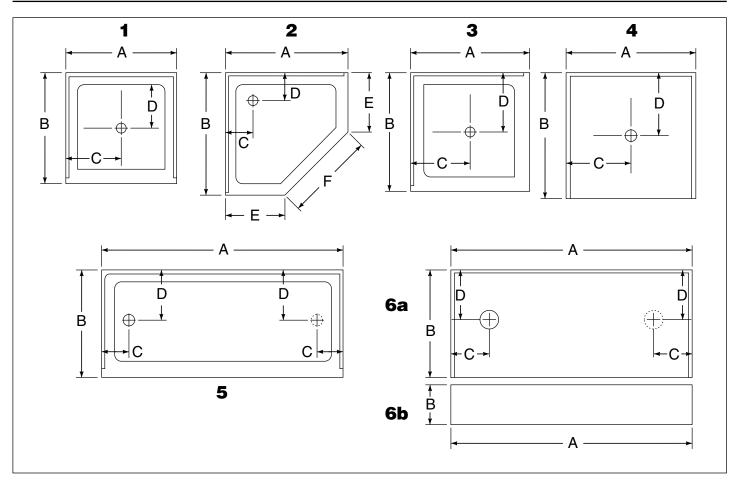
These dimensions are approximate sizes only. For proper fit, measure the actual shower floor prior to building the framework to determine the exact size. Add 3/8" to the width measurement and at least 3/16" to the depth measurement of the actual shower floor to create the size of the framework opening needed.
