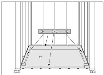
**Note**: Clean up any excess mortar/thinset and allow the mortar/thinset under the barrier-free shower floor ramp to cure for 24 hours.
