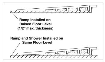
Place the barrier-free shower floor ramp into all eight of the stainless steel clips to prevent the shower ramp from moving. The front (thin) edge of the shower floor ramp must completely contact the floor surface.
