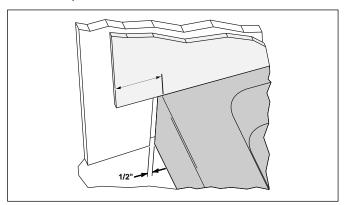
2. Hold the apron strips in place and scribe the angle of the shower base onto each piece. Remember, do not cut the finished edge.
