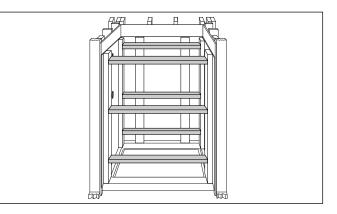
4. Insert small blocks between the front-to-rear panel braces and the back panel braces. These will apply pressure to the back panel to hold it in place.
