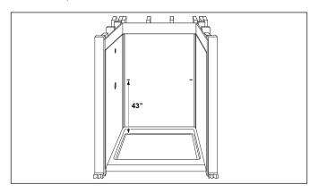
2. After marking the height, draw a 4" level line on both walls. These lines will be used to align the top edges of the soap dish.
