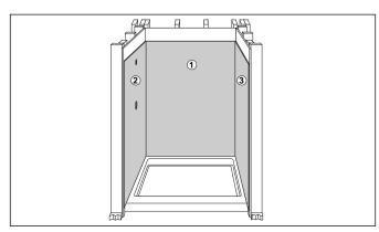
4. Firmly press the surface of each panel against the wall. It is important to apply hand pressure to the entire surface of the panel to bond it to the wall surface.
