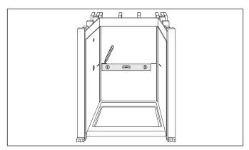
3. Dry fit the soap dish prior to applying silicone. If the wall is not exactly 90 degrees square, it will be necessary to sand the sides of the soap dish in order to achieve proper fit, using a course grit (60 grit) sandpaper.
