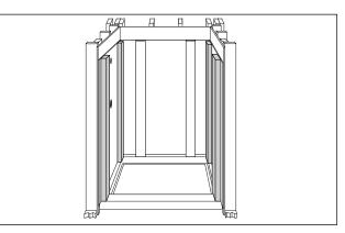
3. Install (wedge) three horizontal braces (six total) against the left and right wall braces.
