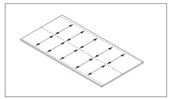
**Note**: The back panel can be cut **slightly** smaller than the opening because the side panels will cover any small gap (less than 1/4 inch).
