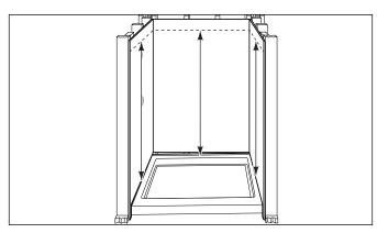
3. Transfer these measurements to both side panels and the back panel. Cut the bottoms of the panels.
