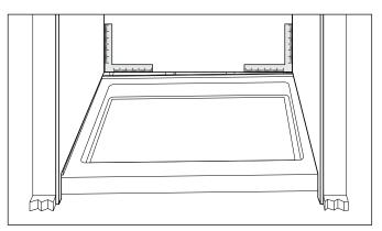
2. If the shower base is not perpendicular to the wall, use a level and draw a line around the alcove on all three walls. Measure the distance from the line to the top of the shower base.
