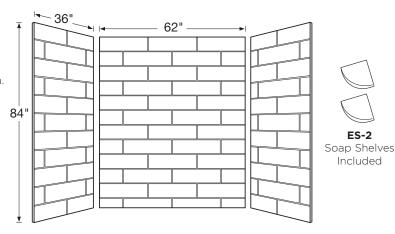
Designed to fit base areas 36" deep or smaller x 62" wide x 84" high or smaller (914 mm x 1575 mm x 2134 mm)
