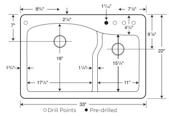
Capacity: 8  $\frac{1}{2}$  gallons in large (left) bowl until it reaches the divider height, 2  $\frac{1}{4}$  gallons in small (right) bowl until it reaches the divider height
