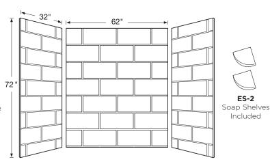
Designed to fit base areas 32" deep or smaller x 62" wide x 72 ½" high or smaller (813 mm x 1575 mm x 1829 mm)
