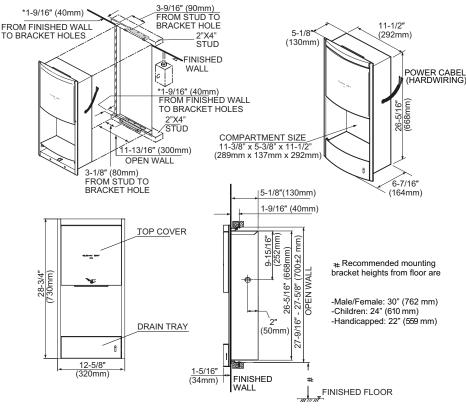
\*WALL THICKNESS REQUIREMENT: MIN 3/16 in (5mm) TO MAX. 1-3/16 (30mm)
