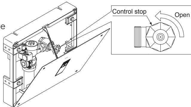
**NOTE:** The control stop should never be opened to the point where the flow from the Flush Valve exceeds the flow capability of the fixture. In case of a valve failure, the water must overflow from fixture.
