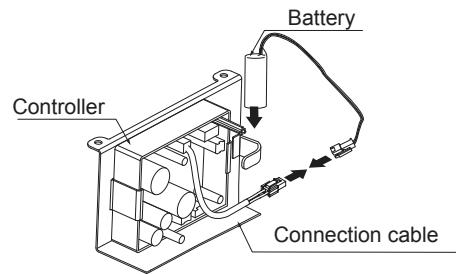
12. Connect the cables of infrared sensor and controller with the connection cable.
