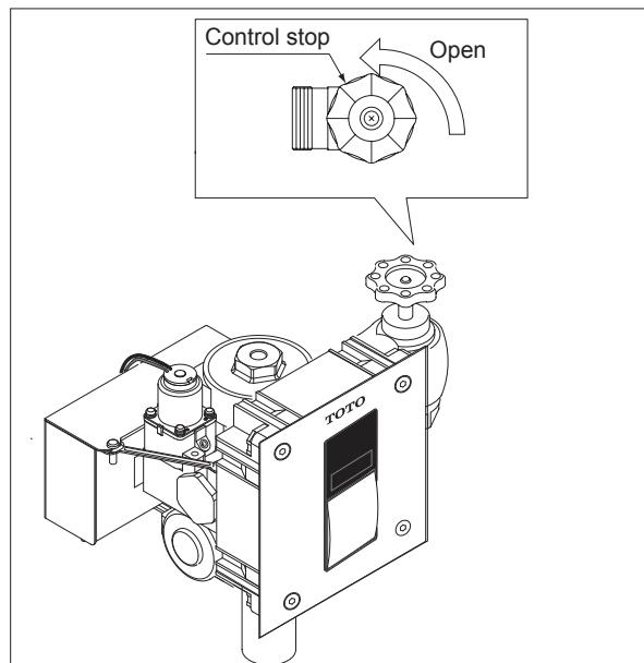
**WARNING:** Do not open the control stop to the point where the flow from the Flush Valve exceeds the flow capability of the fixture. In case of a valve failure, the water must not overflow from the fixture.
