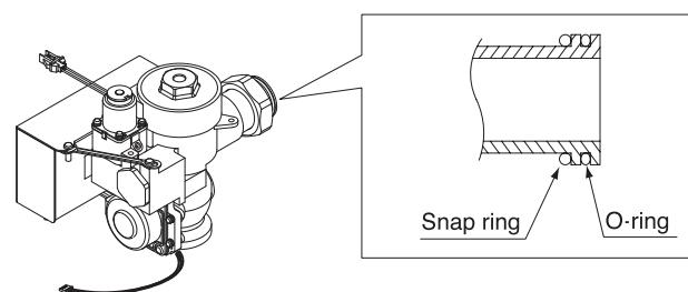
10. Connect the Flush Valve with the control stop and vacuum breaker tube.
