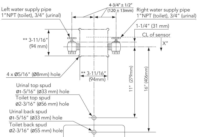
To use with a left water supply, detach the controller and remount it to opposite side of valve body.
