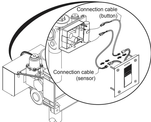
**NOTE:** It will take 5 minutes after connecting the battery for the electronics to initialize. After approximately 30 seconds, the sensor LED will flash in 4 second intervals until the initialization completes.
