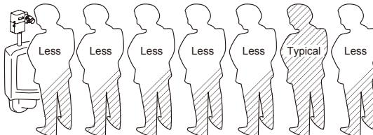
If the idle time is short, the system assumes frequent use and the Flush Valve discharges less water.
