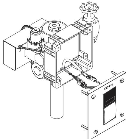
17. Fasten the front cover to the base frame by tightening the screws with the supplied hex wrench.
