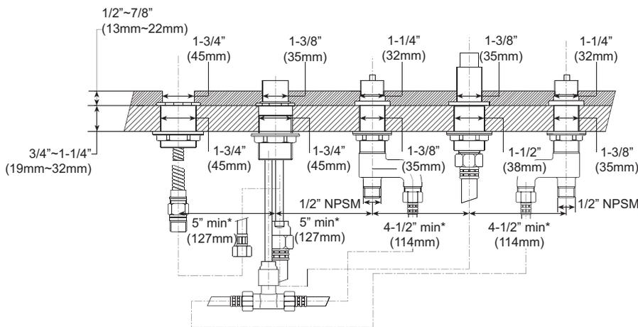
**IMPORTANT NOTE:** This valve/trim can only be installed in a built-up deck. It cannot be installed on pre-finished deck or on tub rim.
