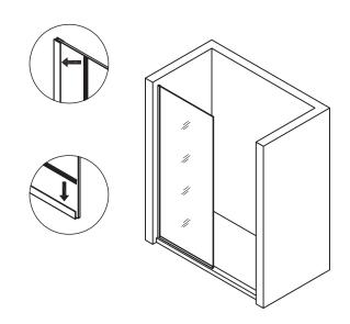
Step 6: Insert wedge gasket Insert the wedge gasket into the gap between glass panel and wall jamb, glass panel and bottom strip.
