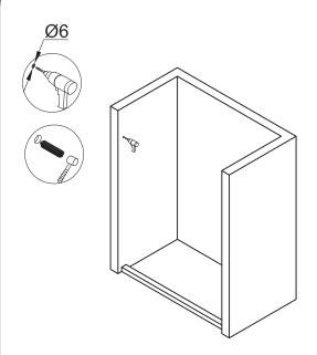
**Step 3: Drill holes**Drill holes onto where marked at last step and put in wall plugs.
