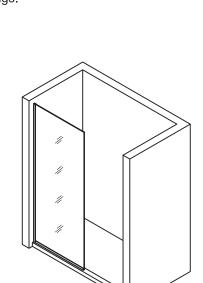
**Step 5: Fit on glass panel**Insert the fixed panel into the wall jamb and the bottom strip.
