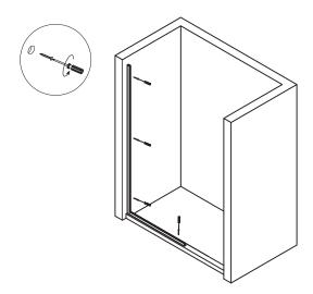
**Step 4: Fix frame**Fixed wall jamb to wall and the bottom strip to the shower tray or bottom base.
