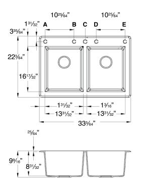
IMPORTANT: Circle Letter(s) above to indicate location(s) for faucet hole drillings (there is a 4" spread between hole locations B,C,D. There is a 10<sup>25</sup>/<sub>64</sub>" spread between hole locations A and B and D and E).
