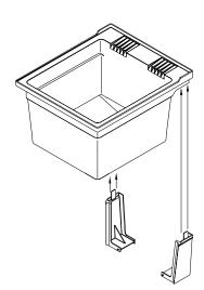
Attach the filler plates to the back of the tub as shown. The tongue on top of the filler plate should fit into the groove under the backside of the tub. The attachment pins on the bottom of the filler plates will align with the holes in the tub. Note that there is a left and right filler plate. If they are not used on the correct side the pins will not align with the holes. The filler plate may need to be tapped with a hammer to push the pin into the hole completely.
